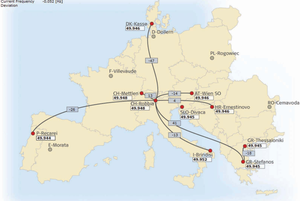
FIGURE 5.22 Swissgrid web page showing current European PDCs links (January 2012). (© 2012 Swissgrid AG. All rights reserved. With permission.)
