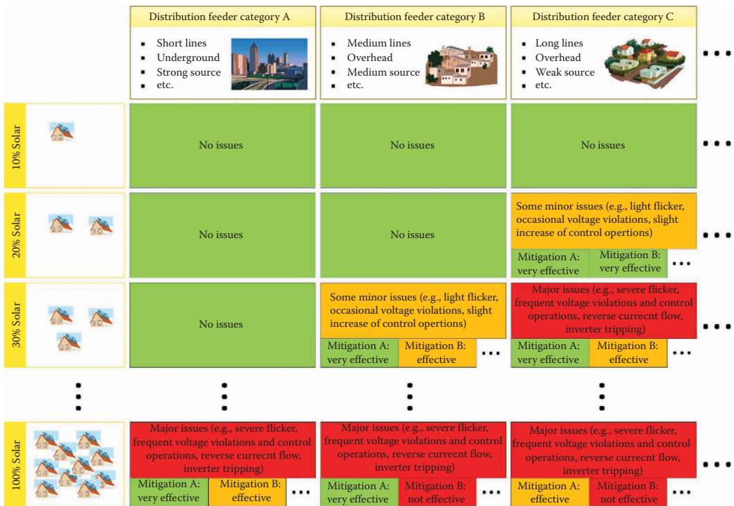
FIGURE 6.16 Solar penetration levels and effectiveness of mitigation options according to distribution feeder categories (conceptual).
