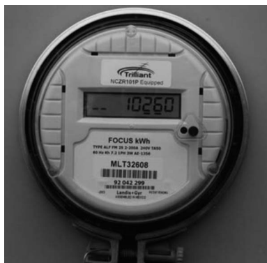
FIGURE 13.2 Example of a solid-state smart meter. (© 2012 Trilliant. All rights reserved.)
