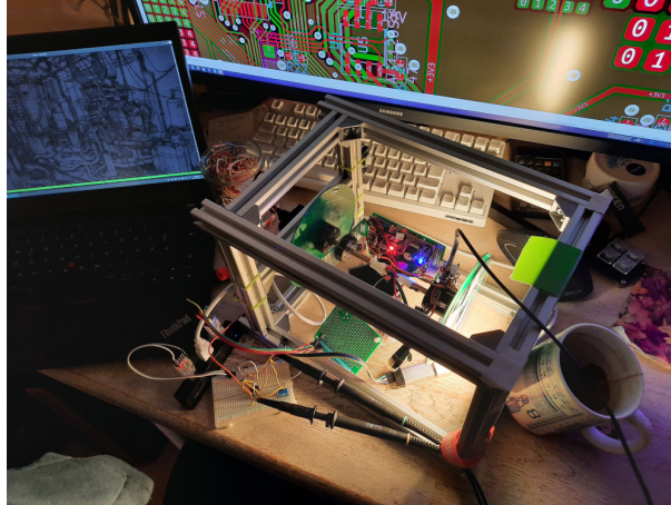
Figure 1: The prototype when we first achieved reliable power transfer and bidirectional communication between stator and rotor. In the picture, the prototype was communicating reliably up to the maximum \approx 1500 rpm that we could get out of its hobby quadcopter parts.
